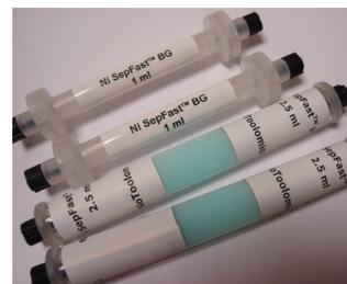
Metal ions are immobilised to the carefully designed porous agarose supports via covalently attached strong chelating groups.
